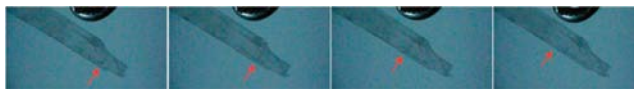
Figure 8. Induction of undulation motions along a crystal twin of TBB by periodic lateral heating (in this figure, the heater is visible on the top right). Note the reversible undulation that can be sustained by approaching the crystal with the heater, as seen by migration of the reflective front marked with red arrows (for details, see Movie S9, SI).
